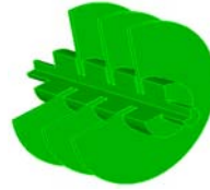
Figure 1: 4-cell iris slot structure.
