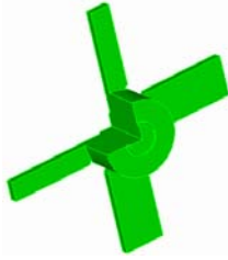
Figure 10: Waveguide damped structure
