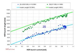
Figure 3: Measured and simulated (solid lines) HER bunch length as a function of a bunch current at the 2S for two different RF voltages: 16.5 MV (blue diamond) and 14 MV (green squares). Measurements were done in multi-bunch regime.
