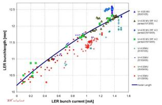
Figure 2: LER bunch length as a function of a bunch
