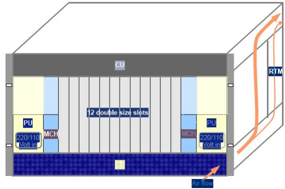
Figure 14: MTCA Shelf 12 AMC Payload Slots Rear IO \mu RTM (Courtesy K. Rehlich, DESY)
