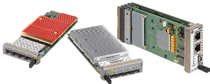
Figure 5: Processor AMC Modules and MCH (Courtesy C. Engels, Emerson)
