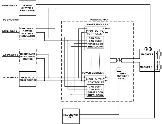
Figure 1 Power System Block Diagram - Redundant Bipolar Operation is Illustrated
