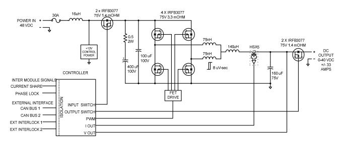
Figure 2 Power Module Schematic Diagram
