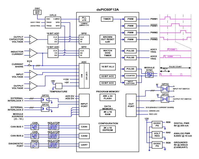
Figure 5 Controller Block Diagram
