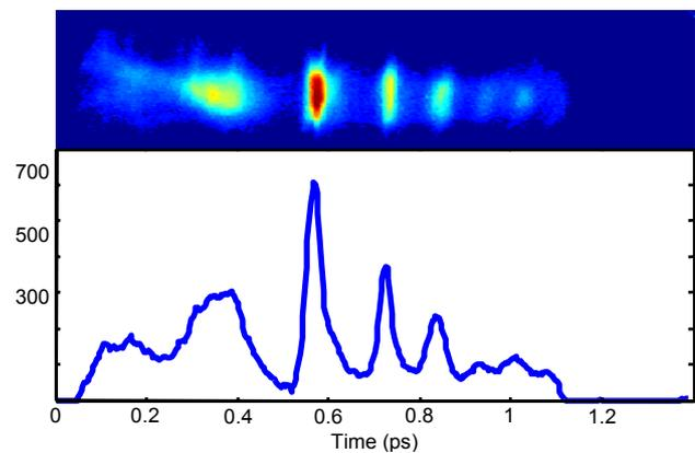
Figure 1: Modulated beam image after spectrometer (upper figure), vertical axes is y-coordinate; horizontal one is proportional to beam energy. Bottom figure: “zero-phasing” projection of the beam on upper plot, horizontal axis is scaled in picoseconds.
