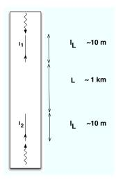
FIG. 2: A diagram of the proposed setup for a terrestrial experiment. The straight lines represent the path of the atoms in the two  $I_L \sim 10$  m interferometers  $I_1$  and  $I_2$  separated vertically by  $L \sim 1$  km. The wavy lines represent the lasers.
