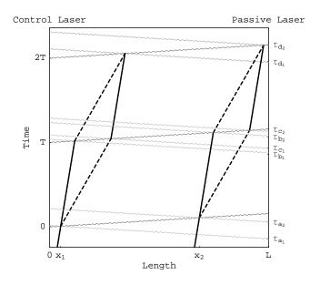
FIG. 1: A space-time diagram of two light pulse atom interferometers in the proposed differential configuration. The black lines indicate the motion of a single atom. Light from the control and passive lasers are incident from the left (dark gray) and the right (light gray) respectively.
