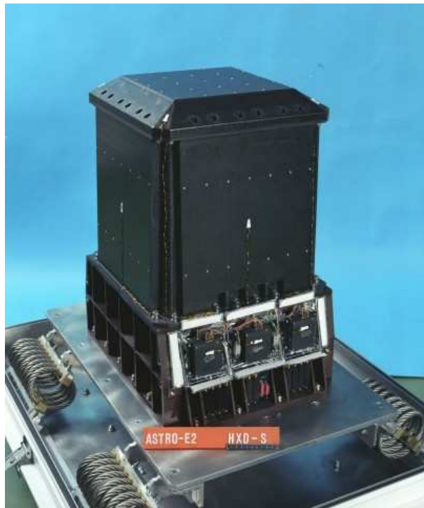
Fig. 1. Hard X-ray Detector before installation.
