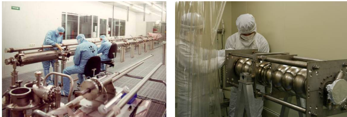
Figure 4: Clean room environments are mandatory. Left: the assembly of eight nine-cell TESLA cavities into a cryomodule string at DESY. Right: an ICHIRO nine-cell cavity is prepared for initial tests at the Superconducting RF Test Facility (STF) at KEK.
