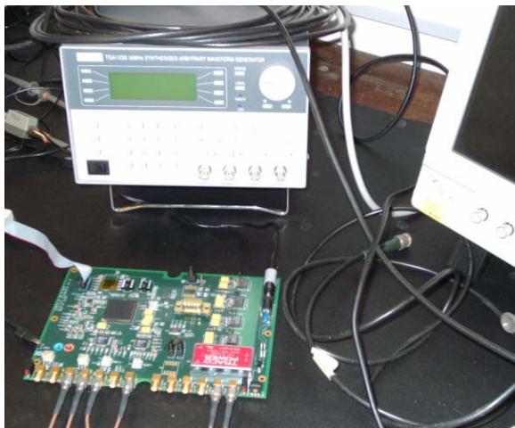
Figure 7: FONT4 digital feedback processor board in bench test.
