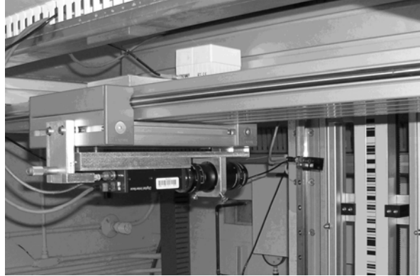
Figure 3: CCD camera set up as part of the SLAC vertical comparator.
