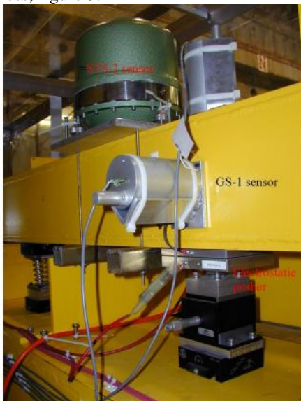
Figure 3: Close-up of sensors and electrostatic actuators.
