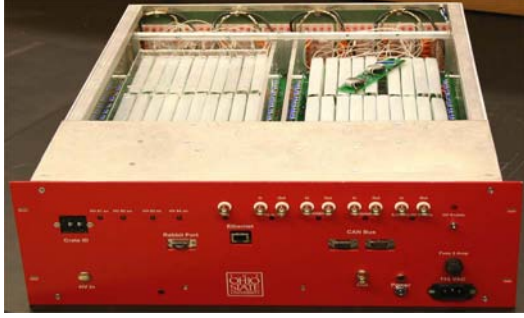
Fig. 1. OSU HVPS with top cover and RF shields removed. One current monitor module has been extracted.
