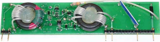
Fig. 2. OSU HVPS current monitoring module.
