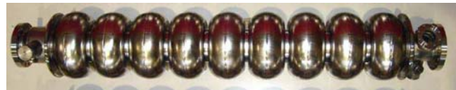
Figure 9: Prototype of ICHIRO cavity under high power processing at KEK with enlarged end-tube shown on the input end to the left.
