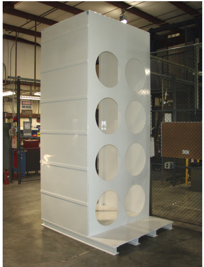
Figure 9. External Casing for the 150kW Test Load.
