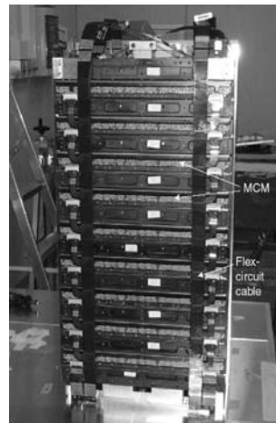
Fig. 1. Inverted view of one tracker module, with a sidewall removed. Nine MCMs and 2 flex-circuit cables are visible.
