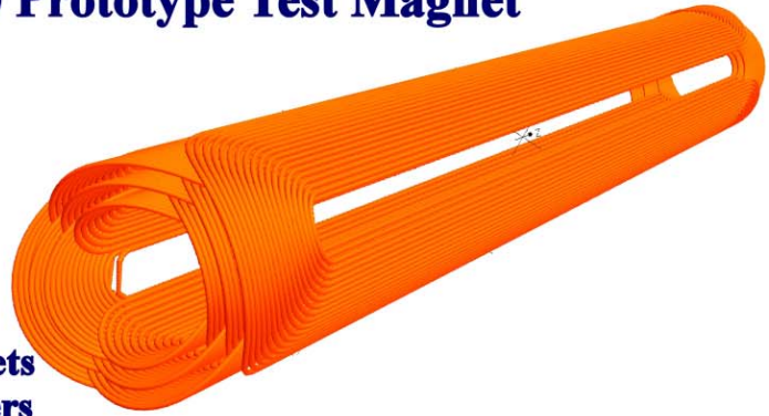
Figure 2: Start of winding for QD0 Prototype Test Magnet, QT, along with 3D view of the final coil configuration.
