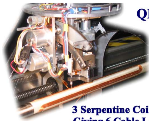
Figure 2: Start of winding for QD0 Prototype Test Magnet, QT, along with 3D view of the final coil configuration.
