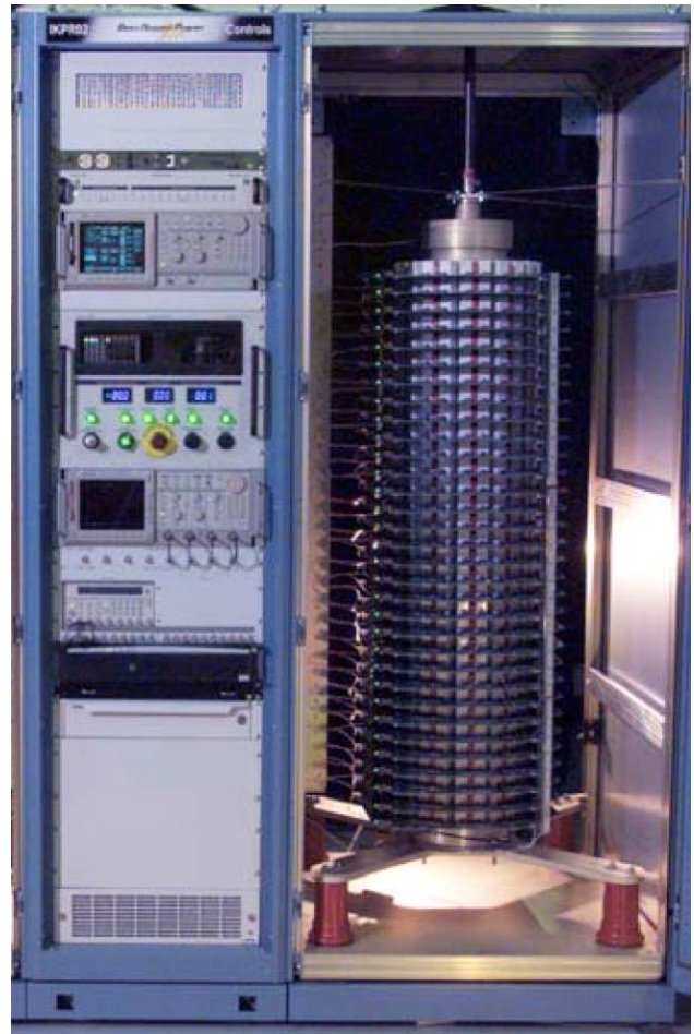
Figure 5: DARHT II Kicker Modulator Assembly
