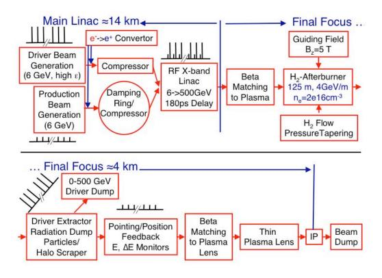
**FIGURE 1.** Flowchart of the RF linac and afterburner. The bunch patterns are also sketched (not to scale). Note that in the actual design the damping ring and compressor are located at the 2 GeV point of the 6 GeV S-band linac. In the present flow chart they are put after the 6 GeV linac for simplicity.
