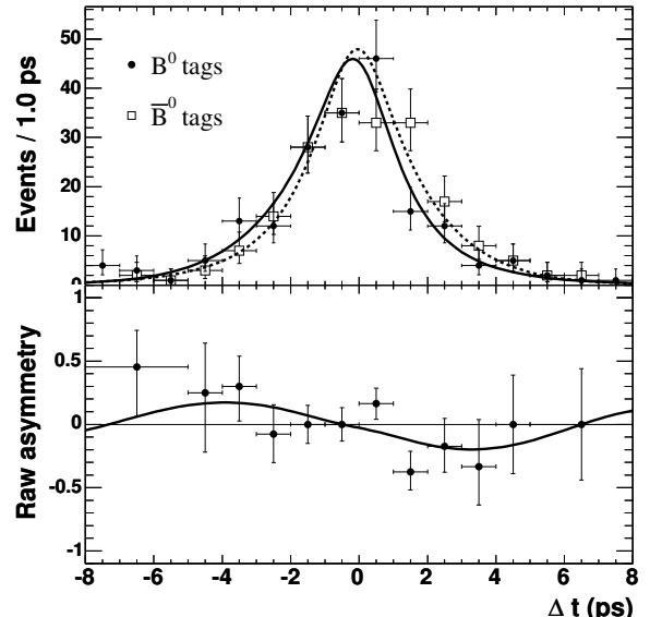
FIG. 2: From top to bottom: the distribution of  $\Delta t$  in the region  $m_{\text{ES}} > 5.27 \text{ GeV}/c^2$  for  $B^0$  ( $\bar{B}^0$ ) tag candidates, and the raw asymmetry  $(N_{B^0} - N_{\bar{B}^0})/(N_{B^0} + N_{\bar{B}^0})$ , as functions of  $\Delta t$ . In the upper plot the solid (dashed) curves represent the fit projections in  $\Delta t$  for  $B^0$  ( $\bar{B}^0$ ) tags.
