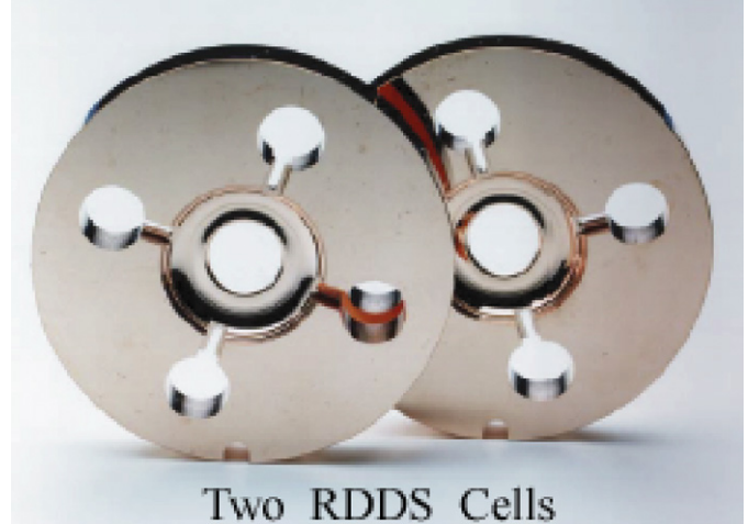
Fig. 2. Rounded damped and detuned NLC type accelerator cell structure.
