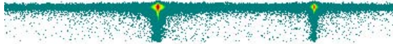
Fig. 10.— Simulation of a set of 10 \text{ \AA} photons. The plot shows the pulseheight vs. dispersion histogram. The left peak is the first order spot and the right peak is the second order spot. Large scattering wings are present off a sharply peaked core along the dispersion direction and the partial event tails of the pulseheight distribution extend vertically. Red represents the high intensity regions, and green represents the low intensity regions.
