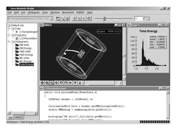
Figure 1 The JAS application showing histogram browsing, plot display, code editor and WIRED event display.
