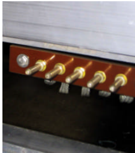
Figure 1. Left: Modulator Tank w/ 5045 klystron, Right: Multi-lam pins for ground
