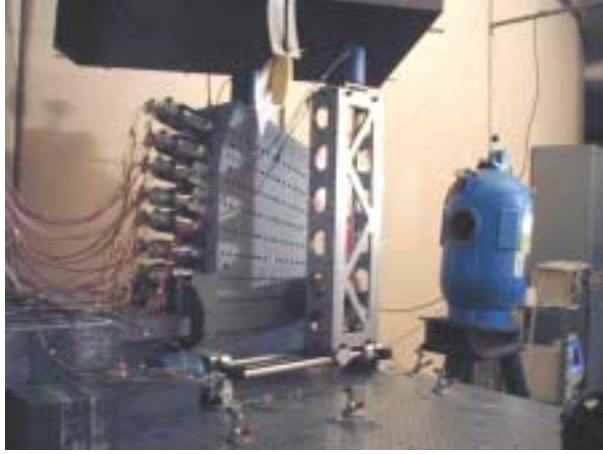
Fig. 1. Experimental Setup: crystal array on the left, ^{60}\text{Co} source on the right.
