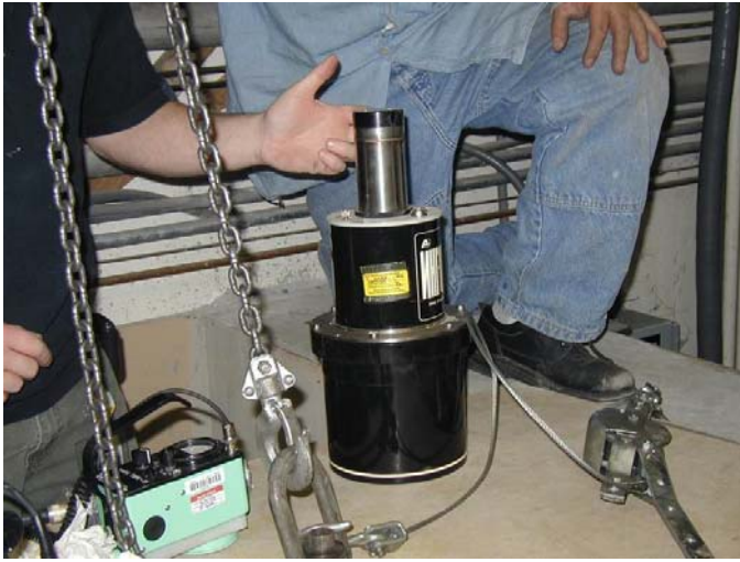
Fig. 3. The neutron-generating unit of the neutron generator system.
