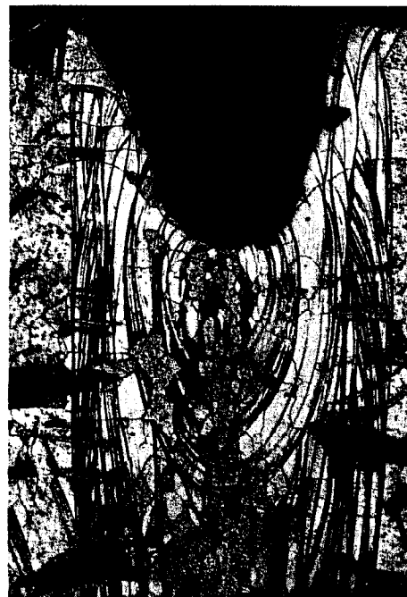
Fig. 9. Parallel-gap welding heads. Fig. 11. Electron beam weld in copper
