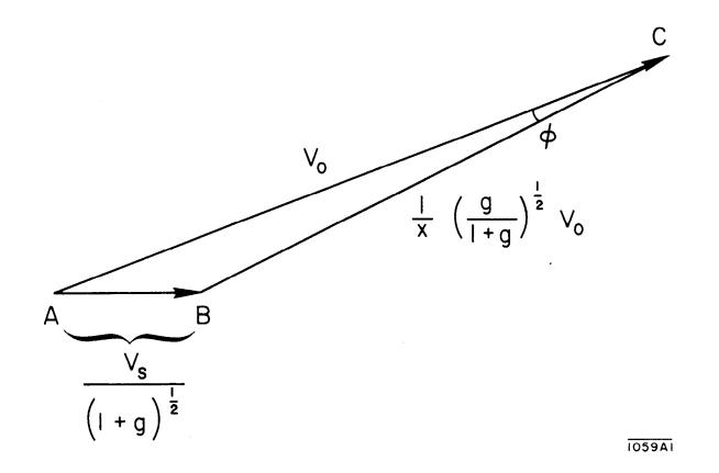
FIG. I STEADY STATE CONDITION IN FEEDBACK LOOP WITH PHASE ERROR  $\phi$  .
