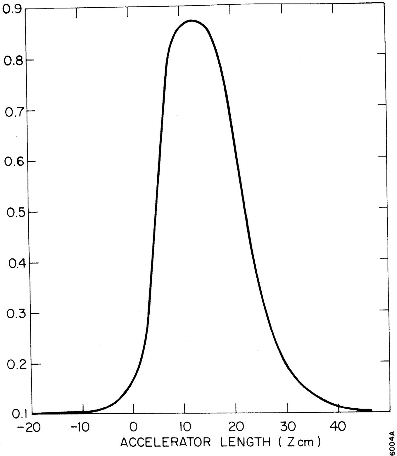
ELECTRIC FIELD INTENSITY IN 10' SECTION AT 4139.6 MHz
