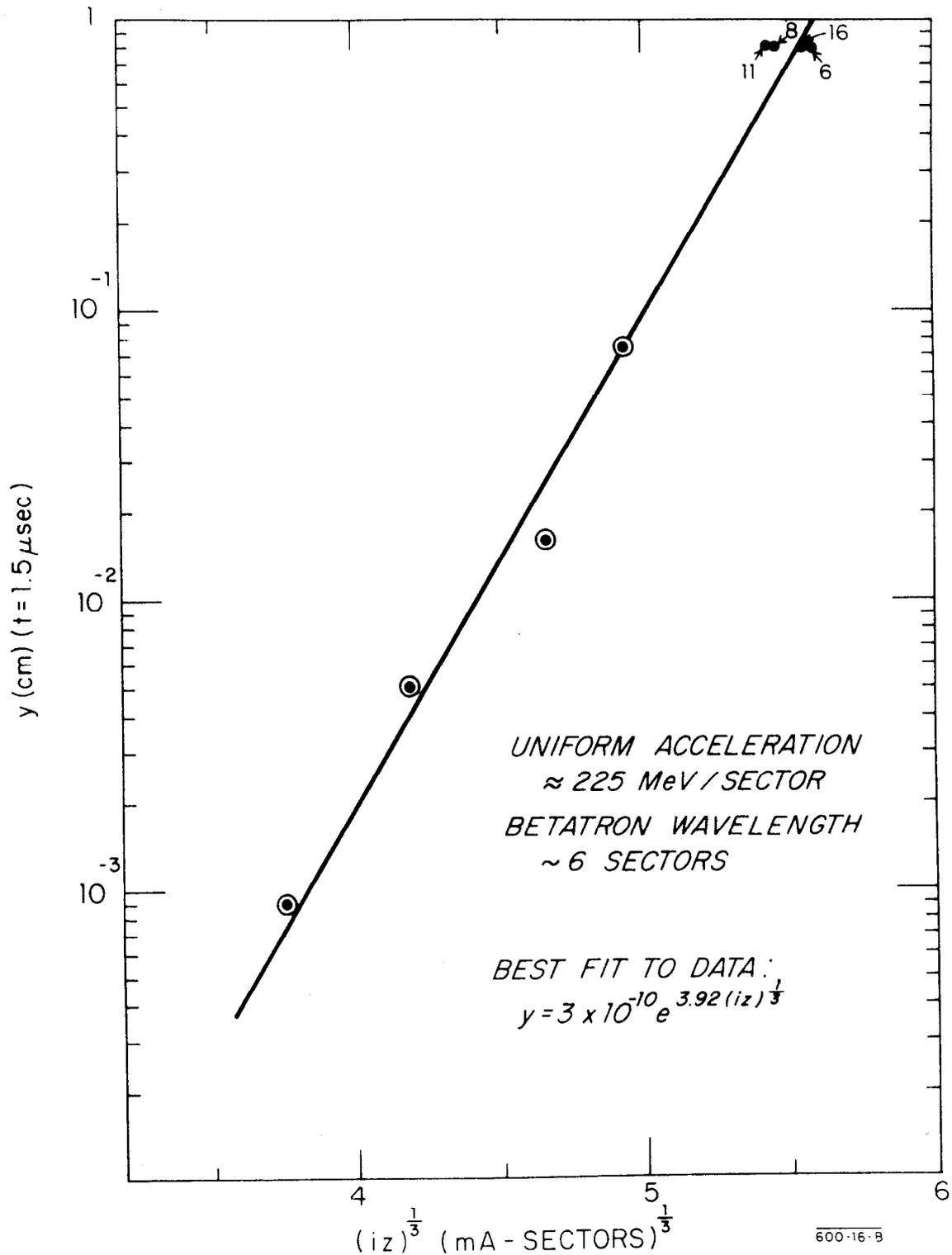
FIG. 11 -- TRANSVERSE MODULATION IN BBU AS A FUNCTION OF  $(iz)^{1/3}$ . CIRCLED POINTS MEASURED BY OBSERVING INDUCED POWER IN C-BAND PROBE AT END OF SECTOR 5. NUMBERED POINTS ARE THE ONSET OF SCRAPING AT SECTOR INDICATED.
