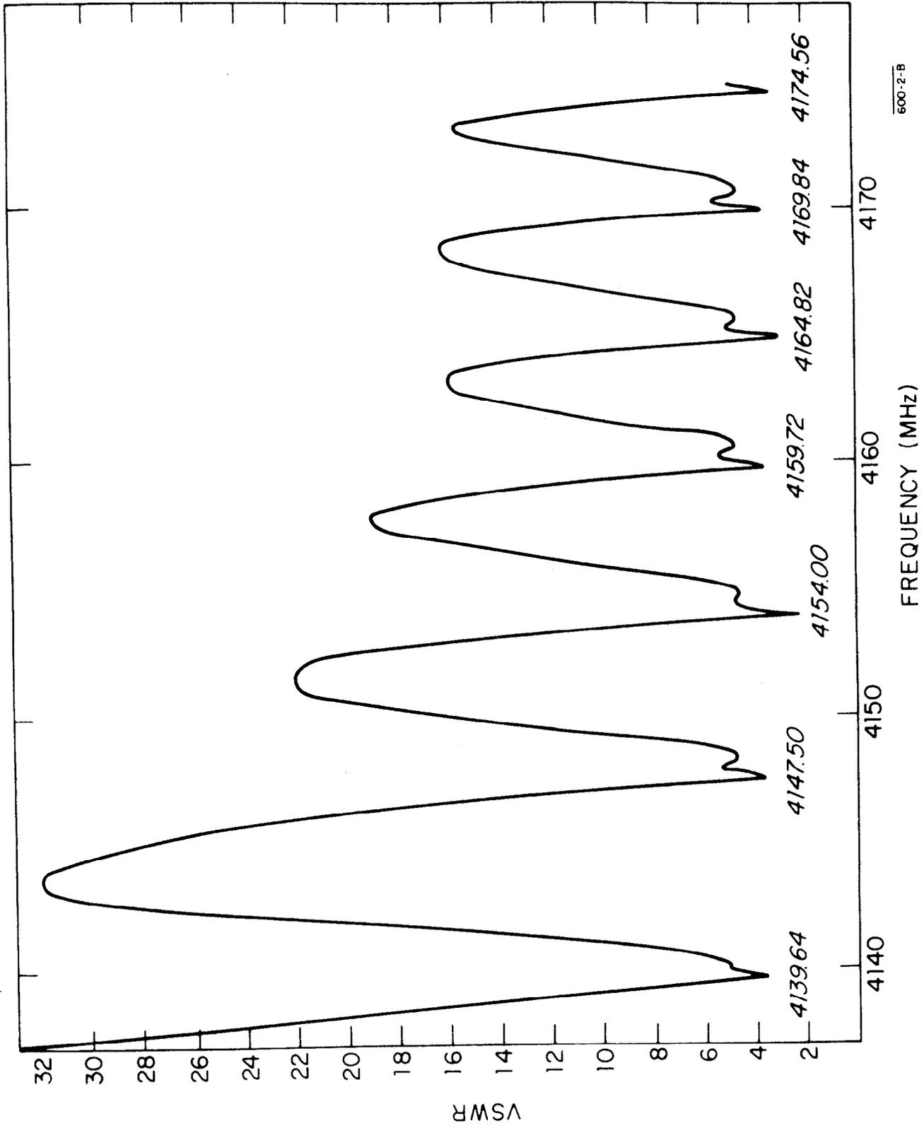
FIG. 15 -- VSWR LOOKING INTO INPUT OF TEN-FOOT ACCELERATOR SECTION
