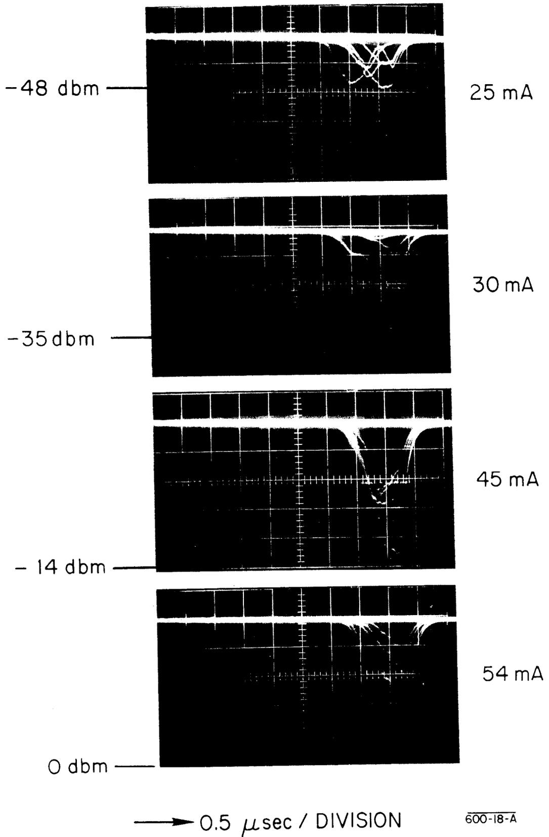
FIG. 20--RF PULSES INDUCED AT 1284 MHz IN
