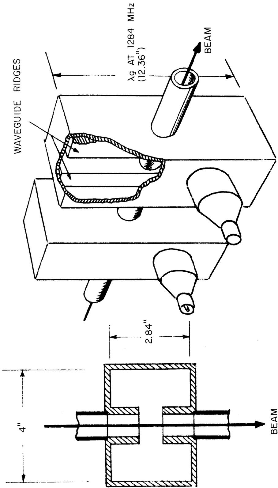
TWIN RIDGED WAVEGUIDE CAVITIES
