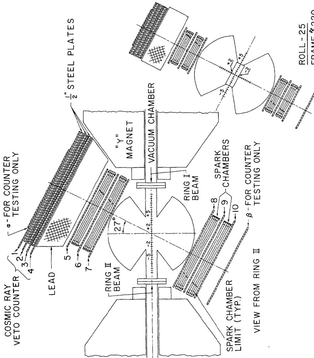
SPARK CHAMBER - COUNTER GEOMETRY
