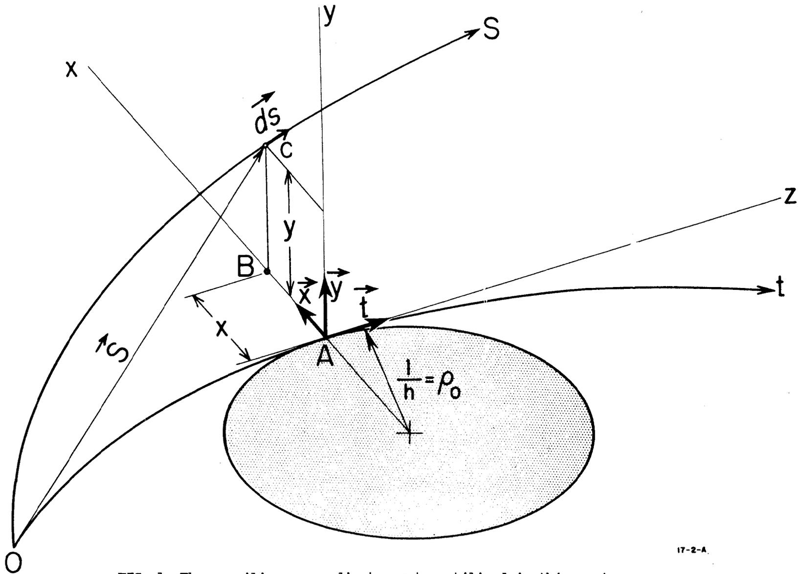
FIG. 1--The curvilinear coordinate system utilized in this system.
