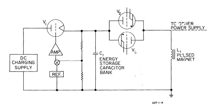
FIG. 1 - BASIC CIRCUIT OF PULSED POWER SUPPLY
