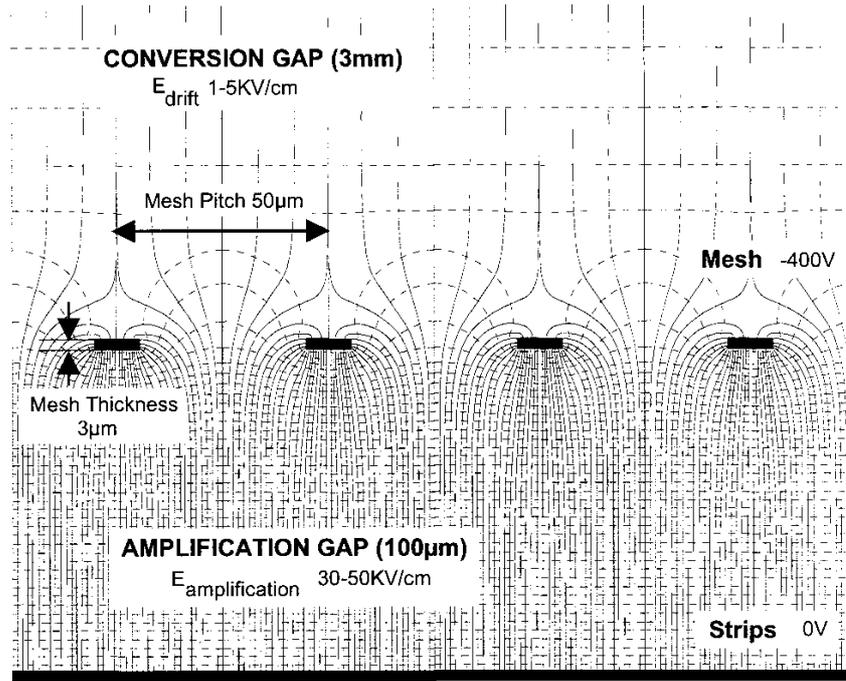
Figure 1. Map of the electric field lines around the micromesh (50  $\mu\text{m}$  step, 37  $\mu\text{m}$  diameter of the openings).
