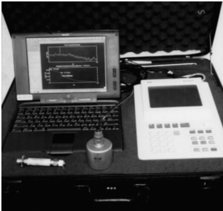
FIGURE 1. Field measurement setup showing the Apple PowerBook 5300c and the Hewlett Packard 3560A Dynamic Signal Analyzer packed in a rolling foam lined suitcase. In the foreground are the pressure transducer and the accelerometer that were used in the measurements.
