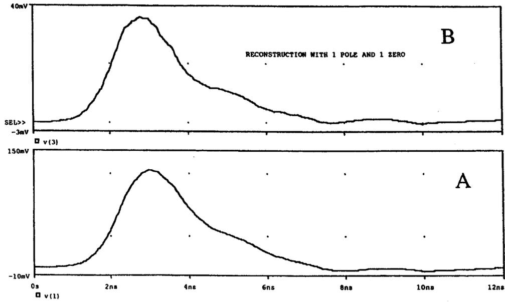
**FIGURE 6.** Signal reconstruction simulation using PSPICE with the “hardware” filter: “A” input signal, “B” output signal after simulated transfer function and filter.
