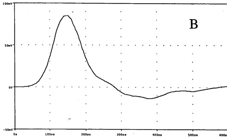
**FIGURE 5.** Signal reconstruction using PSPICE: “A” from the oscilloscope, “B” from PSPICE with simulated transfer function.
