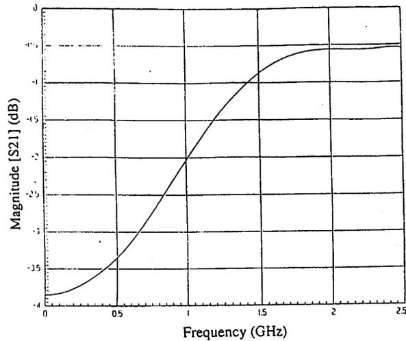
**FIGURE 2.** Simulated transmission coefficient vs. frequency
