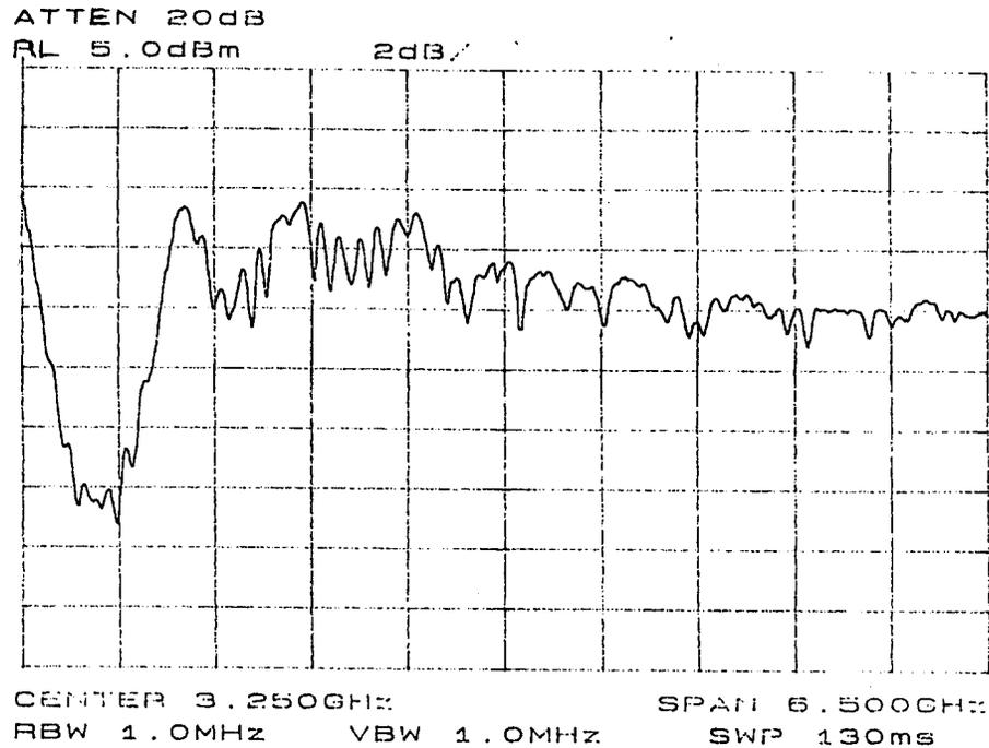
**FIGURE 4.** Frequency response of the TSFFC (range 0–6.5 GHz)
