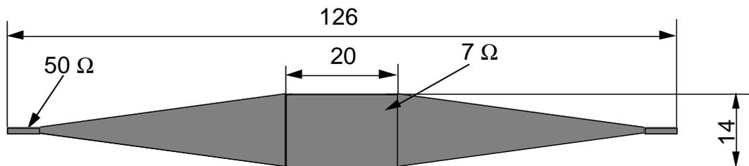
**FIGURE 3.** Fast Faraday Cup dimensions (in mm).
