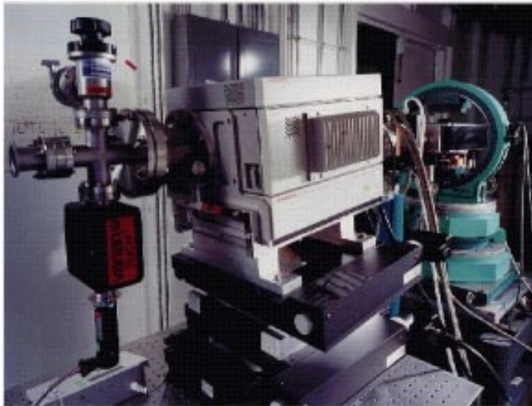
FIGURE 2. A photograph of the x-ray streak camera mounted on the three translation stages for x -, y -, and z(t) -axis motion. The front window is a Be. The streak tube vacuum is obtained with the external ion pump.
