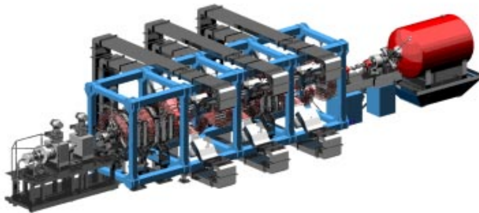
FIGURE 2. The first LEDA experiment configuration that includes the 75 keV injector, the 6.7 MeV RFQ, a short HEBT, and a 670 kW beamstop, is shown.
