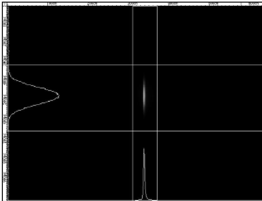
**FIGURE 1.** Typical single-axis streak image for bunch-length measurements, accumulated over many turns. Vertical: 1 ns full scale. Horizontal: position (channel number) along slit. The projections onto the axes, in the regions bounded by cursors, are shown along the sides.
