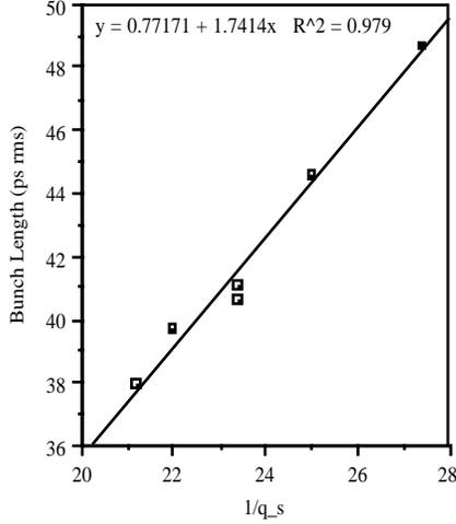
**FIGURE 3.** Variation of bunch length with the inverse of the synchrotron tune, for a single bunch at 1 mA.
