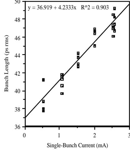
**FIGURE 4.** Variation of bunch length with single-bunch current, at 14 MV of rf; 1 mA corresponds to  $4.6 \times 10^{10}$  electrons in the bunch.
