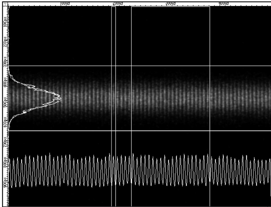
**FIGURE 2.** The light from a single bunch captured on consecutive turns. Full scale: 1 ns vertical, 500  $\mu$ s horizontal. The projections on the left show a single bunch and the sum of the 20 bunches (determined by the two sets of cursors).
