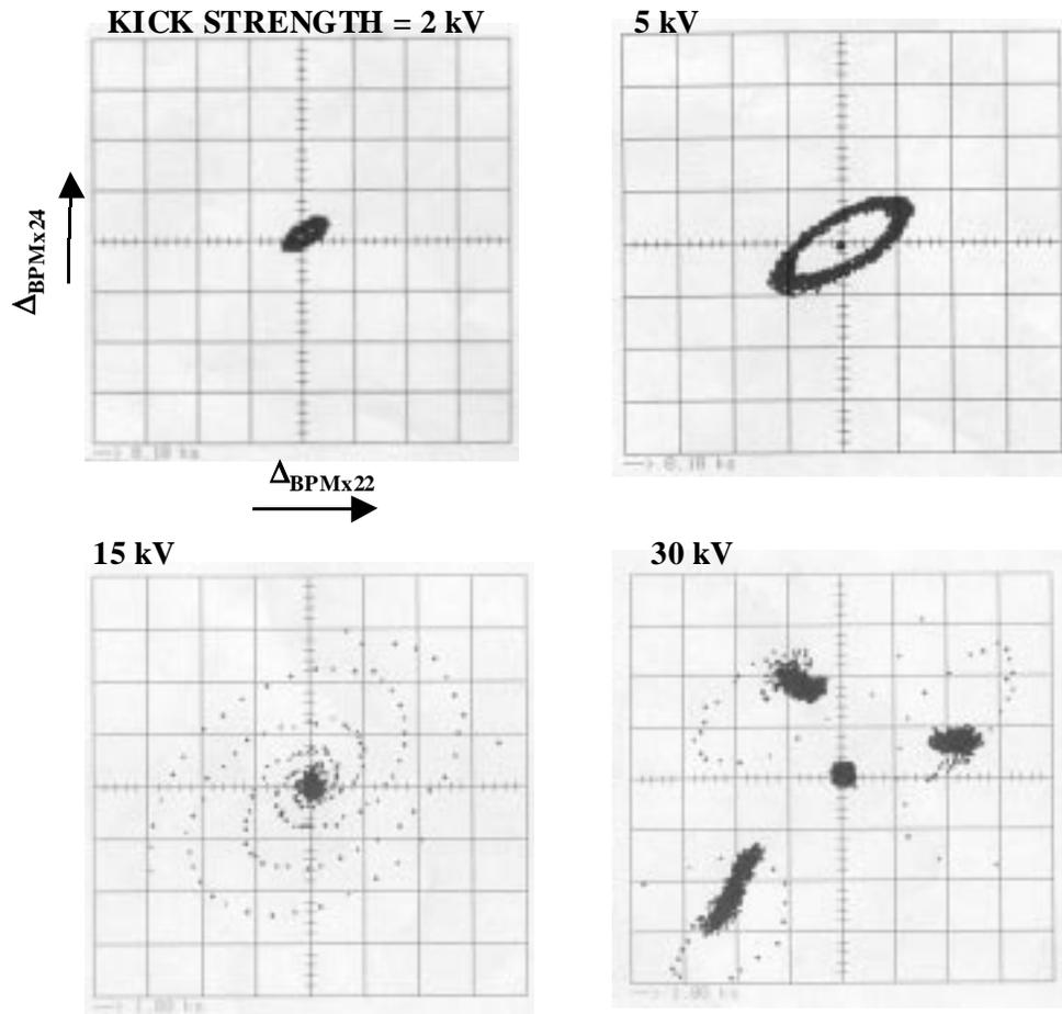
**FIGURE 2.** Horizontal “phase space” plots of an electron-cooled beam at four different kick strengths in kV (deflection angles) displayed on line with a digital storage oscilloscope in  $xy$ -display mode. Vertical direction: analog difference signal of  $\text{BPM}_{x24}$ , horizontal direction: analog difference signal of  $\text{BPM}_{x22}$ .
