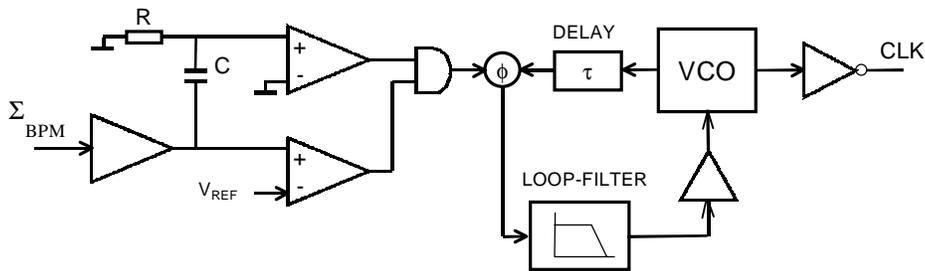
FIGURE 1. Bunch-synchronous tracking generator.
