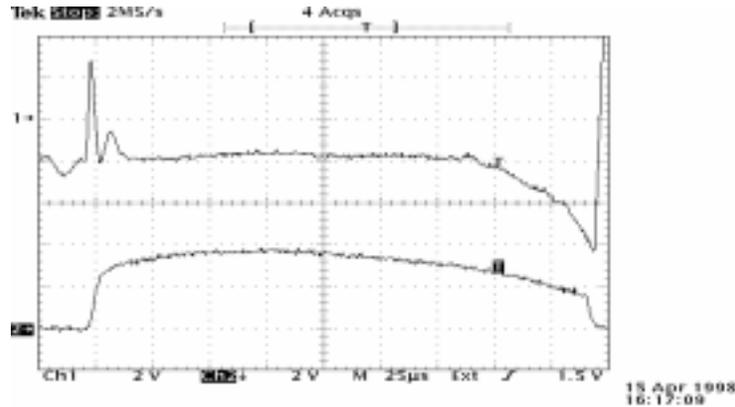
**FIGURE 1.** Top display is the ToF. The average energy is 7 MeV. The bottom display is the CIS stop located downstream of the first dipole. The energy sag at the end of the ToF pulse corresponds with the sag in intensity on the stop.
