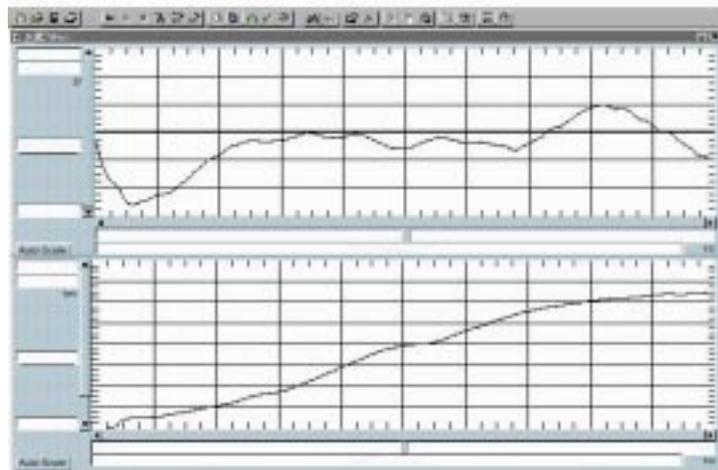
**FIGURE 3.** The upper display is the beam position (2 mm/Div.) in the CIS ring during a 7 MeV ramp. The bottom display is the intensity during the same ramp.
