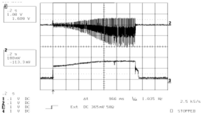
**FIGURE 4.** The top display is the WGM output during a 225 MeV ramp. The bottom display is the output from a logarithmic amplifier of the same ramp.
