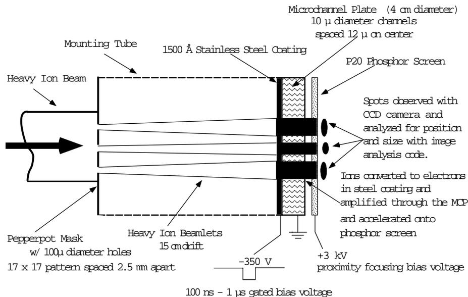
**FIGURE 1.** Schematic view of GBI.
