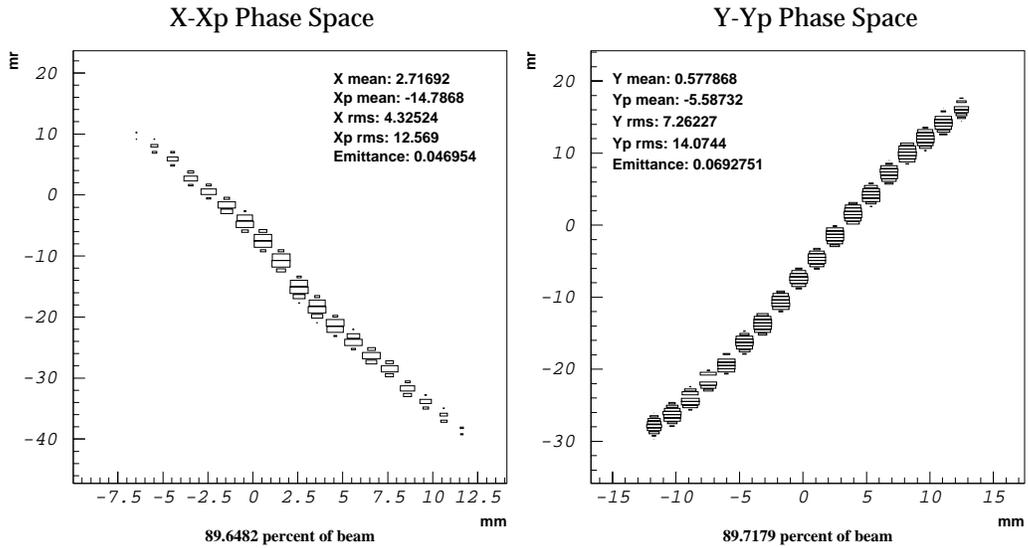
**FIGURE 3.** Slit Scanner results.
