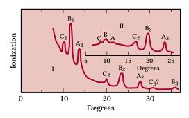
One of the earliest examples of X-ray spectroscopy. The Braggs made a seredipitous discovery: while studying the scattering of X rays off of crystals they noticed that a distinctive pattern of peaks appeared for each of the different anti-cathodes being used to produce the rays. What had initially started out as a study of the structure of crystals led to an investigation of the atomic structure of the anti-cathode elements. [Bragg and Bragg, PRS, 88A, 413 (1913).]
