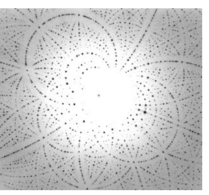
White radiation Laue diffraction pattern from the protein trimethylene dehydrogenase (an enzyme that catalyzes the conversion of trimethylamine to dimethylamine and formaldehyde) recorded on SSRL beam 10–2 with a 5 msec X-ray exposure. The photograph was taken by Scott Matthews and Scott White of Washington University, St. Louis, and Mike Soltis, Henry Bellamy, and Paul Phizackerly of SSRL/SLAC.
