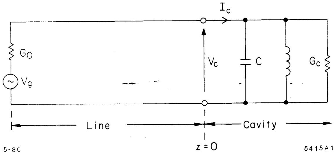
Figure 1. SLED equivalent circuit
