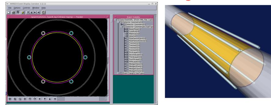
6-8 external lines Reduced material (no water jacket) No coating, gold foil only Non-homogeneous temperature distribution Non-homogeneous material thickness
