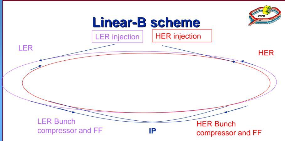
Overall ring length about 6Km, Collision frequency about 120Hz\*10000bunch\_trains=1.200MHz
