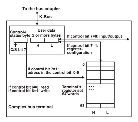
The control or status byte occupies the lowest address of a logical channel. The corresponding register values are located in the following 2 data bytes. (The BK2000 is an exception: here, an unused (reserved) data byte is automatically inserted after the control or status byte, and the register value is therefore placed on a word boundary).
