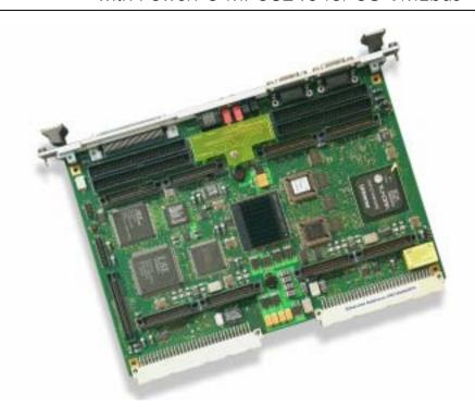
The VIPC824x is an intelligent 6U VMEbus carrier board with four IndustryPack (IP) slots with front I/O, NVRAM/RTC, a highly integrated MPC8240 PowerPC™ microprocessor with an MPC603e CPU kernel, 32MB RAM, a powerful DRAM controller, and PCI interface. The combination of a MPC8240 processor and IndustryPack slots provides a powerful CPU and a modular I/O solution for applications in process control, telecommunication, medical systems and traffic control.
