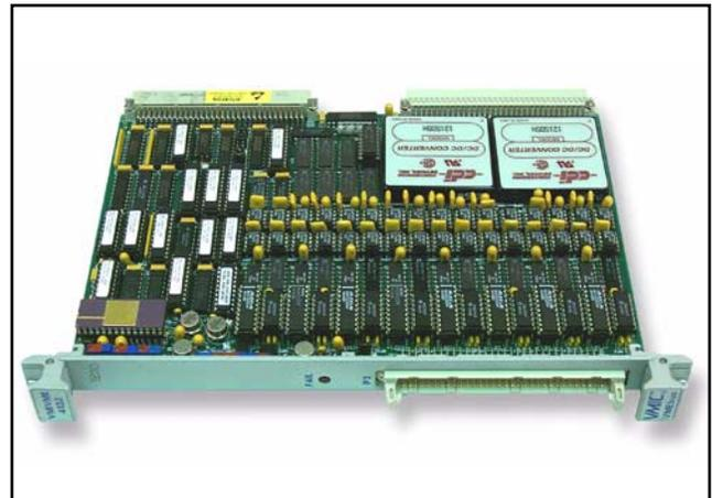
**Built-in-Testing:** Built-in-Test logic provides the user with the capability to test all of the active components on the board, including the output switches. This test scheme utilizes an on-board analog-to-digital converter (ADC) and multiplexers, as shown in Figure 1.
