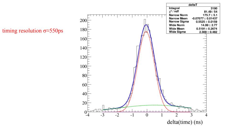
Run 27, position 1, 3M triggers/119k good single tracks in CAMAC stream
