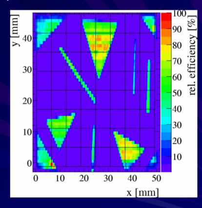
Made scans with pads #5,7,8 connected to hi-res Phillips 7186 TDC for detailed x,y crosstalk studies.
