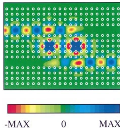
FIG. 5(color). Electric field pattern of the structure shown in Fig. 2 at the resonant frequency. The white circles indicate the position of the rods.
