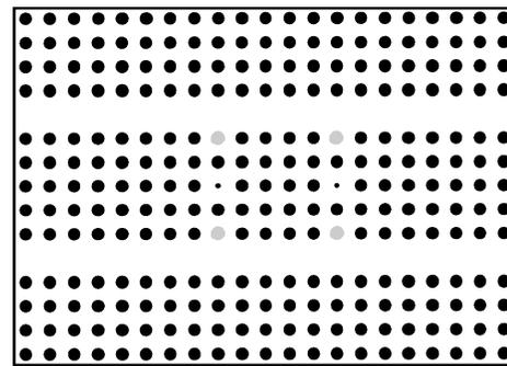
FIG. 2. Photonic crystal structure with two waveguides and two cavities. The black circles correspond to rods with a dielectric constant of 11.56, while the gray circles correspond to rods with a dielectric constant of 9.5. The two smaller rods have a dielectric constant of 6.6, and a radius of  $0.05a$ , where  $a$  is the lattice constant.
