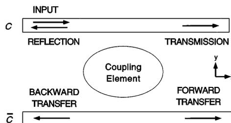
FIG. 1. Schematic diagram of two continuums coupled through an element which supports localized resonant states.
