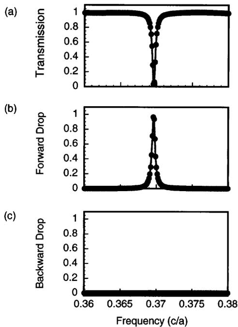
FIG. 4. (a) Intensity spectrum of the transmitted signal in the structure shown in Fig. 2. (b) Intensity spectrum of the transferred signal in the forward direction. (c) Intensity spectrum of the transferred signal in the backward direction. The solid dots are obtained from computer simulations. The lines result from analytical theory.
