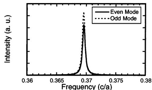
FIG. 3. Spectrum of the even and odd modes for the structure shown in Fig. 2.
